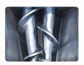
Conical twin screw force feeder
